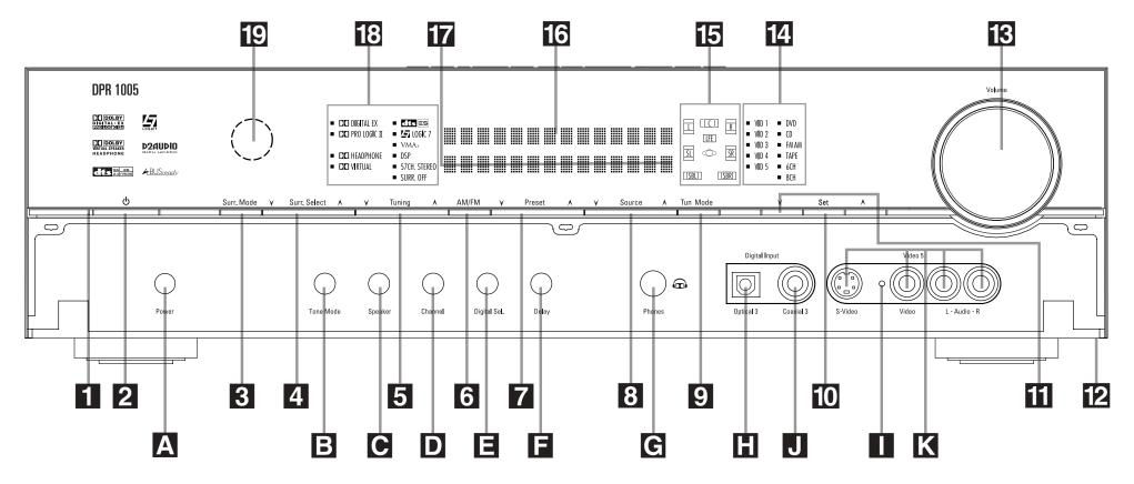
The following controls and indicators are available on the DPR 1005's front panel:
